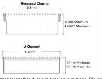
Grates longer than 1500mm supplied in sections. Tile Inserts longer than 1200mm supplied in sections. Channels over 3000mm supplied in sections with joiner. +/-2mm tolerance on dimensions.
